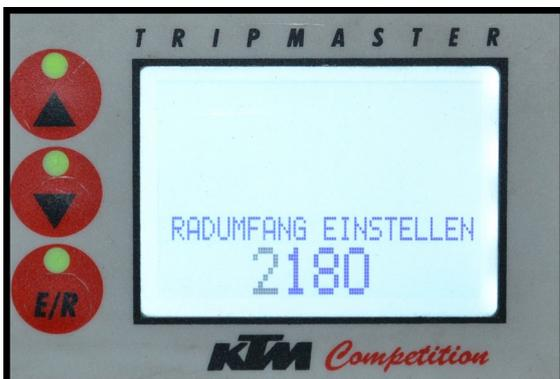
**Step 4:** After you skipped through the wheel circumference setting, you can now set the odometer, e.g. after replacing the internal battery. Please note: This is the value in kilometers, even if you are using the 'miles' setting, you still have to enter the value in kilometers, not miles! Multiply your mileage by 1.61 to convert it to km.
